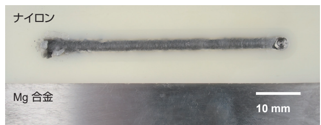
(a) 良好な継手(900 rpm/60 mm・min -1 )
