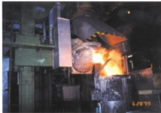
図8 出湯状態 Fig.8 Tapping from GF converter to transfer ladle
